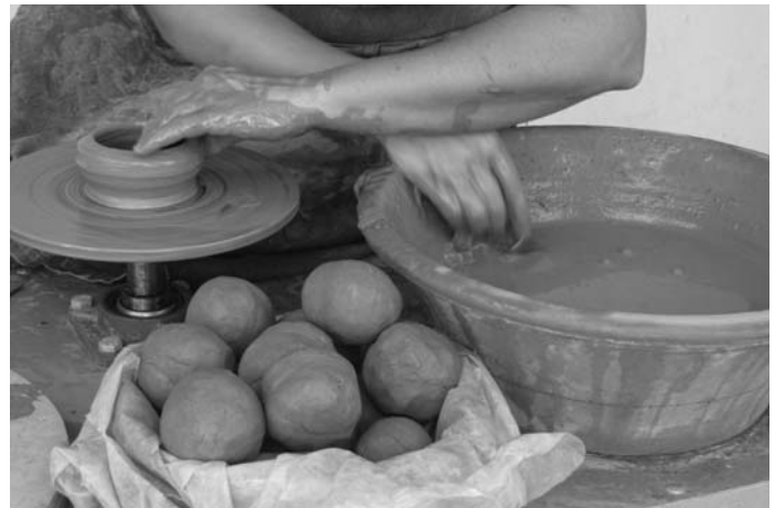
Figure 4. Throwing Mochlos clay on the wheel using slip-slurry. Photograph by S. Kaminis.
